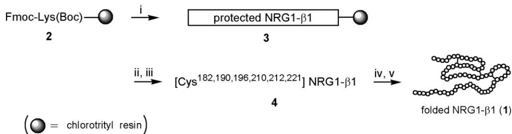
Scheme 1 Reagents and conditions: (i) Fmoc protocol on automated peptide synthesizer (ABI 431A); (ii) TFA/EDT/TIS/H 2 O (94:2.5:1.0:2.5), 90 min; (iii) preparative HPLC (a linear gradient of CH 3 CN in 0.1% aqueous TFA); (iv) overnight stirring in a buffer (Tris-HCl (50 mM, pH 8.0), EDTA (1 mM), GSH (1 mM), GSSG (1 mM)) at rt; (v) preparative HPLC (a linear gradient of CH 3 CN in 0.1% aqueous TFA).
